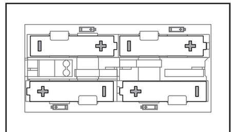
3. Insert the battery case and lock the battery door. Make sure white dot at same side as shown in the picture.
